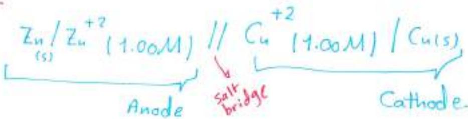
→ The salt bridge is usually a tube that is filled with standard electrolyte soln. such as KCl, KNO<sub>3</sub> --- etc and the purpose of it is to compensate the ions migration by providing the soln. that has a cation migration by cations.
