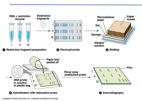
since the probe is radioactive, it will make marks on the Xray plate after placing of Xray plate over the membrane for several days.
