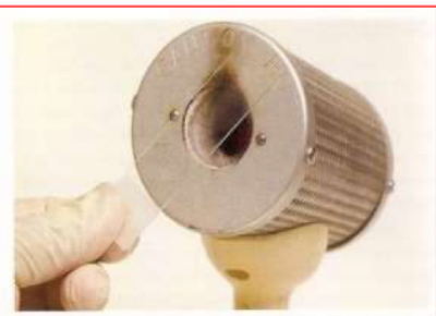
FIGURE 7-40 Heat-fixing a bacterial smear using an electric incinerator
