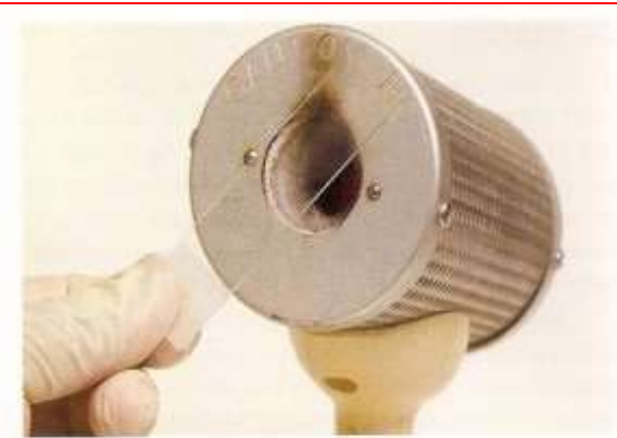
FIGURE 7-40 Heat-fixing a bacterial smear using an electric incinerator
