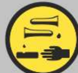
Corrosive Material Hazard
