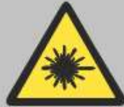
Laser Beam Hazard
