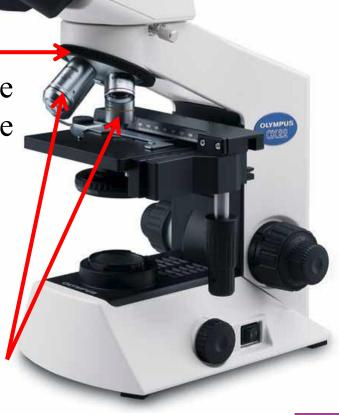
*Total Magnification = Eyepiece power X Objective Lens power*
